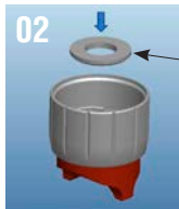
2.- Place the washer inside the aircap
